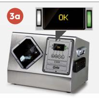
If the container content is identified as acceptable, the **OK message** and a green light are displayed. A short "double beep" is emitted by the internal speaker.
